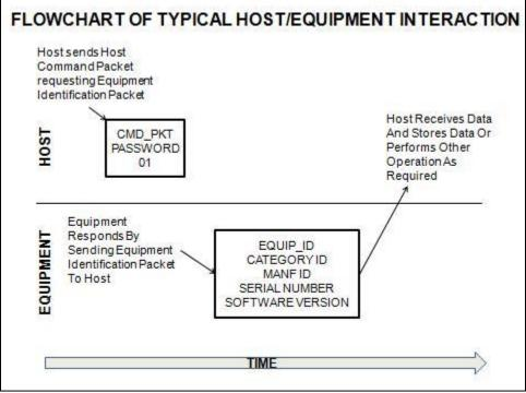
Figure 1- Flowchart Of Host/Equipment Interaction
